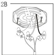
Strip 3/4?of insulation from wire ends. Connect house ground wire to fixture ground wire marked with symbol. Twist wires together using wire nut. Connect black house wire to the fixture wire marked 掛? Twist wires together using wire nut. Connect white house wire to the fixture wire marked 抱? Twist wires together using wire nut.
