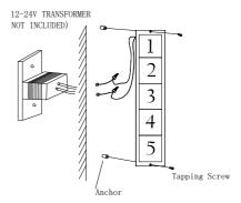
Step 4: turn the light back to front, and wiring the White wire to neutal of power supply, Black wire to Live of power supply.
