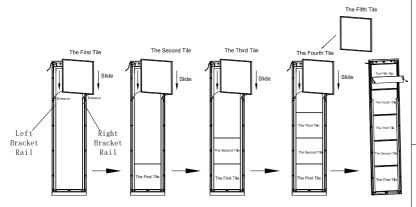
Step 2: As above left, slide the first number into, from the entrance of left bracket rail and right bracket rail between, and then gradually slide down the rest of all number tiles one by one. Finally, screw on the bracket to fix the fourth and fifth number tiles as above right insturction.
