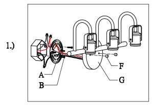
Step.1:Remove mounting bracket (A) from fixture and install to electrical box. Then wire fixture to wires in outlet box. Copper wire is for Ground. Attach backplate(G) to mounting bracket(A) and screws (A1), then tighten by finial(F), so fixture meets wall.
