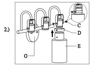
Step.2: Attach metal ring(D) and glass (E) to yoke and secure using set screws(C).
