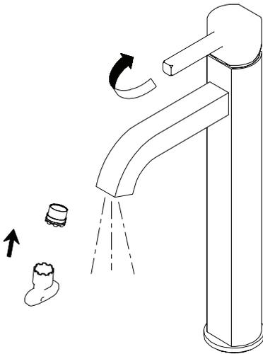
After installing the faucet, remove the aerator (6) with the included aerator key (10). Turn on the water to remove any leftover debris, then reassemble the aerator (6)
