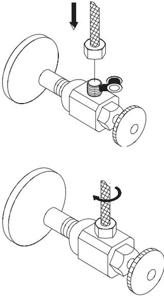
Install flex water supply lines on the angle stops and tighten with an adjustable wrench. Turn on both the cold and hot main valves
