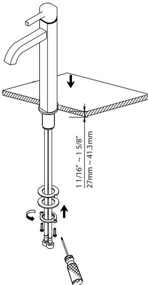
Install the faucet through the 1-3/8" predrilled hole in the countertop. Attach rubber washer (8A), metal washer (8B), mounting nut (8C), and mounting screws (8D) on the threaded mounting pipe. Tighten the mounting nut (8C) until snug. Tighten screws (8D) on the mounting nut (8C) with a Phillips head screw driver until snug
