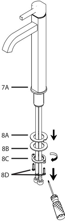
Remove rubber washer (8A), metal washer (8B), mounting nut (8C), and mounting screws (8D). Keep the base trim ring (7A) and rubber washer (7B) on the base of the faucet
