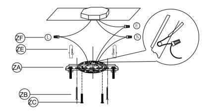
1. Drill two holes on the ceiling and put the plastic anchor screw(ZE) into the holes(If the wall is wood made, this step can be ignored);
